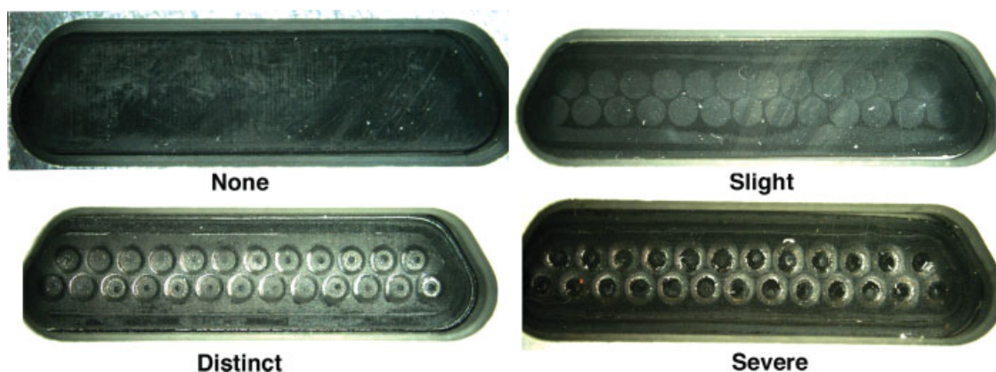
Figure 3 Compression patterns of retrieved gaskets. [Color figure can be viewed in the online issue, which is available at www.interscience.wiley.com .]
